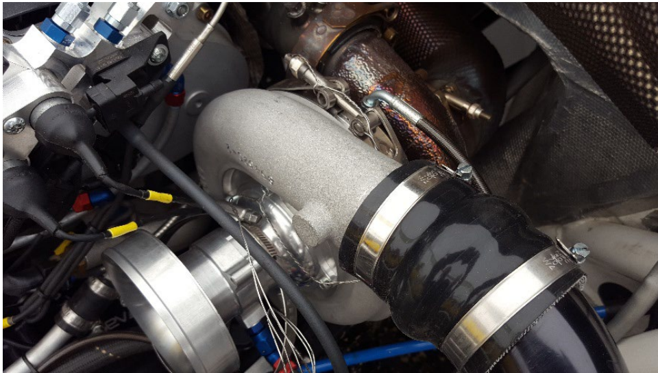
Correct, the wire will start from one point and end after the last bolt (the wire will not make a loop)
